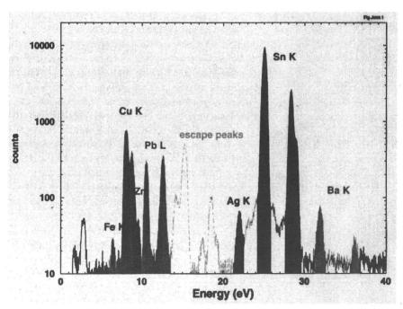
Figure 5. Elemental analysis of Judaidah figurine showing peaks corresponding to tin (Sn), copper (Cu), and lead (Pb). By Ercan Alp, Liz Friedman, and colleagues at Argonne National Laboratory
