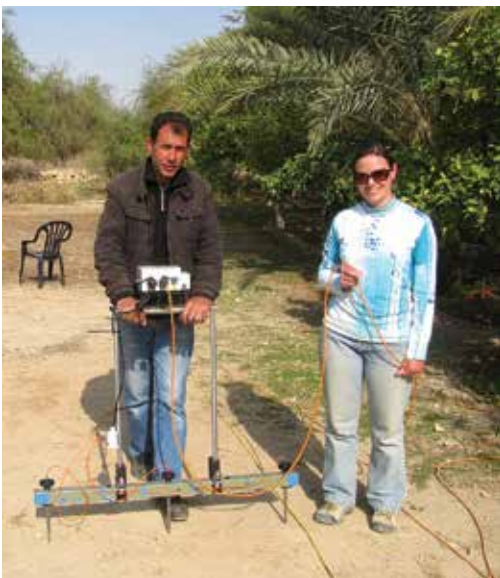
Figure 4. Ellie and Basam using the resistivity instrument in RS 8
