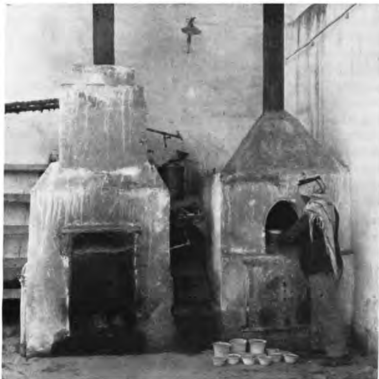
FIG. 38.—Tablets packed in pots filled with sand are being placed in the kiln. The water-heater is shown at the left. Between the two heaters is seen part of the crude-oil burner.
