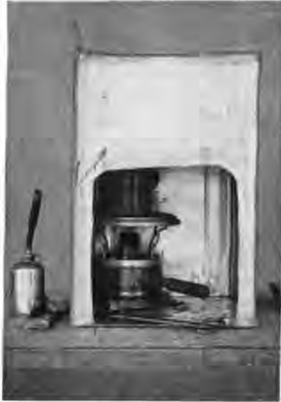
FIG. 35.—Apparatus for heating paraffin in the open air
