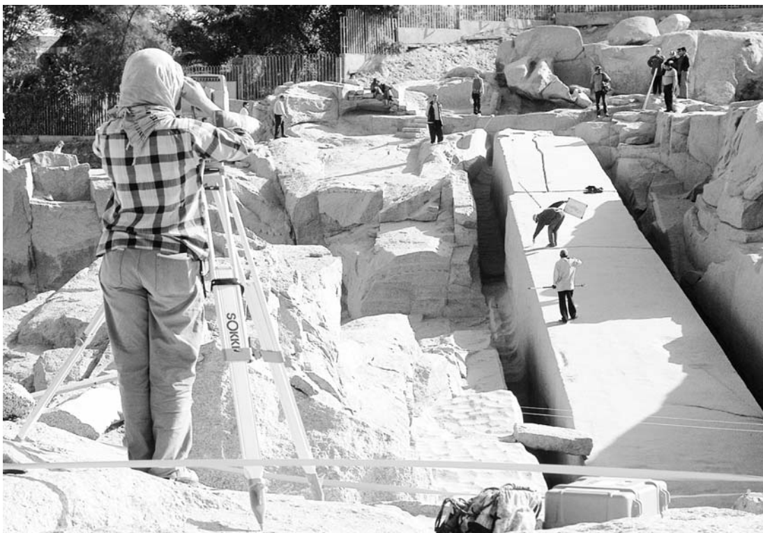
Figure 5. Members of the Giza Plateau Mapping Project surveying in the Aswan obelisk quarry with the Supreme Council of Antiquities. In the foreground Ana Tavares works with the total station
