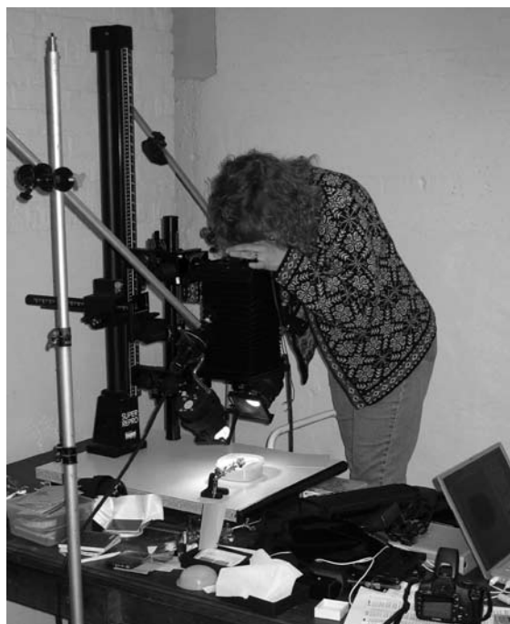
Figure 9. Marilyn Lundberg records Aramaic Persepolis Fortification tablets with large-format, very-high resolution camera and cross-polarized light
