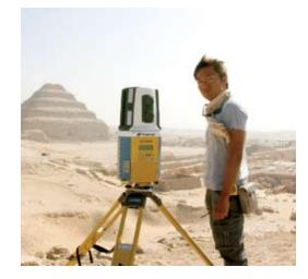
Figure 12. Yukinori Kawae, who organized the SLSS for AERA, at one of two Topcon GLS-1000 laser scanners that the team used for the preliminary overall survey of the Djoser Step Pyramid
