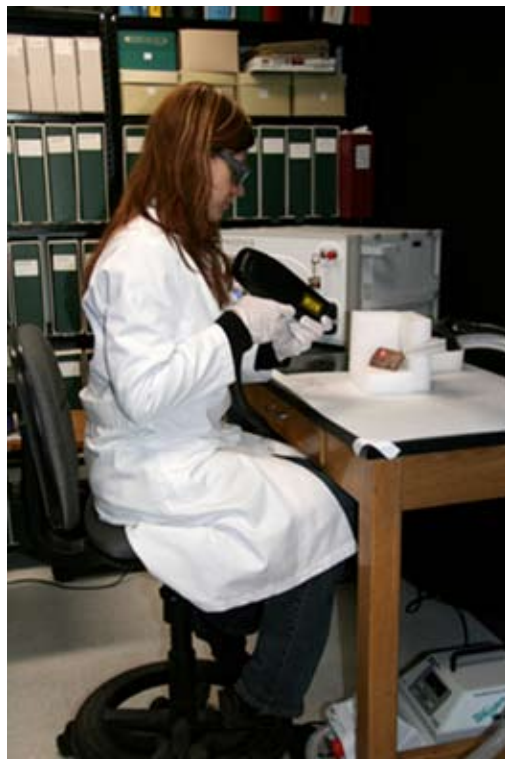
Figure 7. Conservator Monica Hudak cleans a Persepolis Fortification tablet with the Compact Phoenix laser, a.k.a. the "Death Ray"
