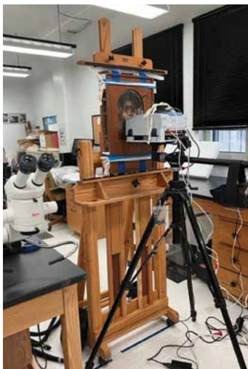
Figure 9. Female funerary portrait undergoing Fourier-transform infrared spectroscopy to aid in identifying materials and pigments.
