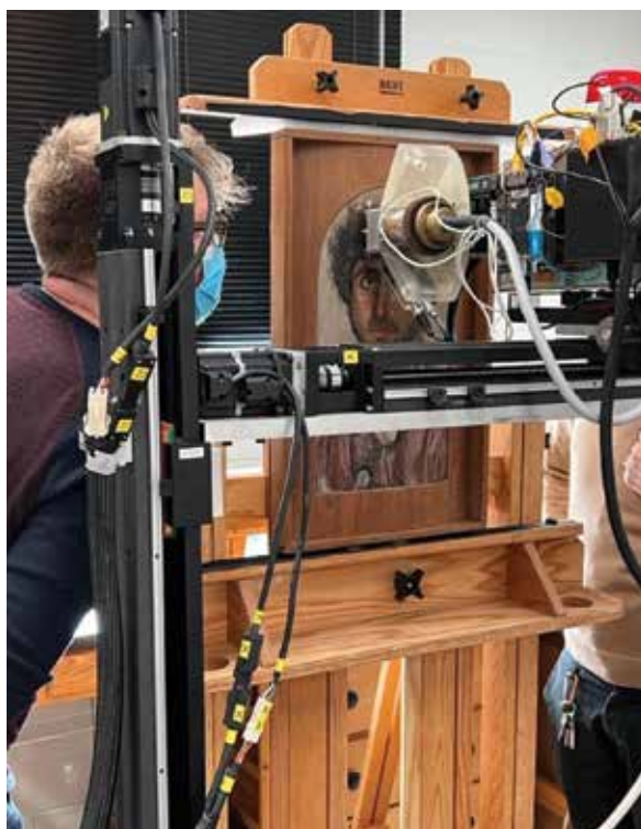
Figure 8. Scientists analyze the surface of a male funerary portrait (OIM E2053) using customized macro X-ray fluorescence equipment to obtain information on the painting's elemental composition.
