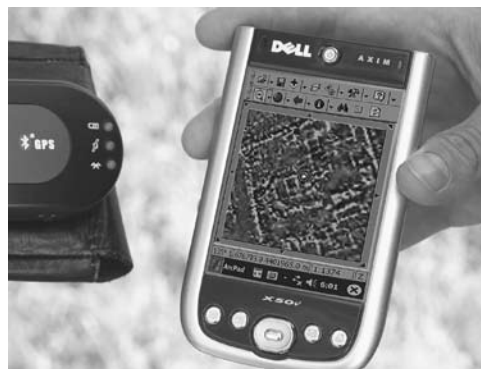
Figure 6. Using a Dell Axim Pocket PC computer and connected Mobile Crossing GPS receiver team members can now walk around the site and see what lies buried directly beneath their feet
