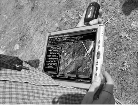
Figure 5. Ground-truthing with the GPS-enabled tablet PC. The GPS allows users to see themselves in real time within the imagery (a small gray circle in the center) and where they are relative to buried structures or streets. The tablet computer also allows users to draw directly on the screen to produce plans of the urban architecture in the field. This same system also works in a vehicle, just like an onboard car navigation system, to allow project members to drive along the network of buried city streets
