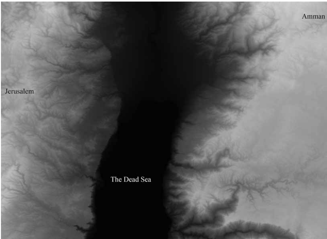
Figure 2. A portion of one of the GDEM Version 2 tiles that CAMEL received from the USGS this year. It shows the topography of the area around the Dead Sea, including the area of the cities of Jerusalem and Amman. Digital Elevation Models are a very useful way to bring elevation information into Geographic Information Systems (GIS) software programs for generating viewsheds, least-cost paths, or 3-D models
