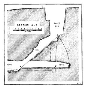
Fig. 22.—Section Showing Eastern Tunnel (1845) and Inclined Passage (1116)
