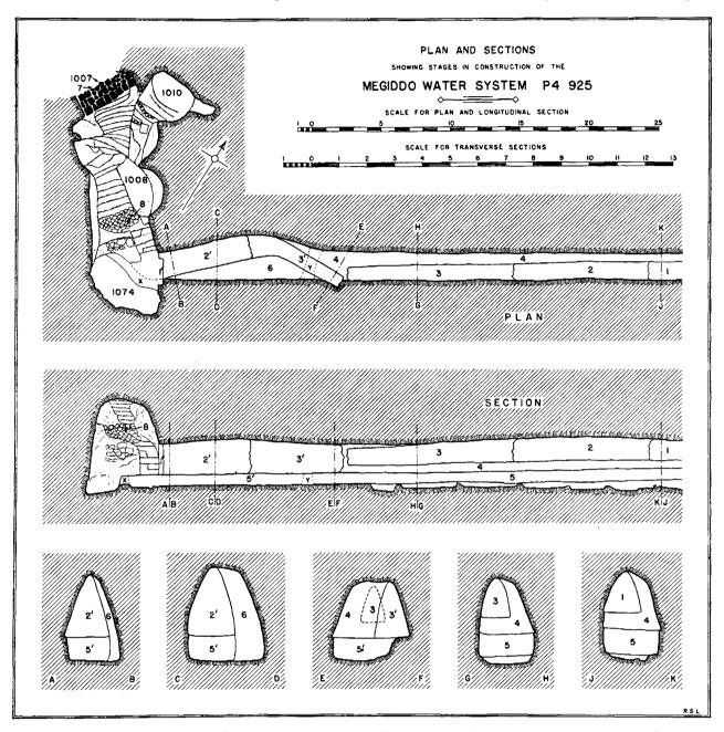
$F_{1G}$ . 13.—Plan and Sections Illustrating the Various Stages in the Construction of the Tunnel. Scale, 1:300 (Transverse Sections, 1:150)
