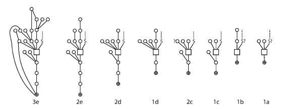
Figure 4.3. Access diagrams of the houses shown in figure 4.2. Rooms within the houses are shown by open circles, and outside space with a cross within a circle. Interconnections between spaces are shown with lines, and the staircase leading to the roof or possible upper story with an S. The square represents the roughly square-shaped room present in all houses, corresponding to the central hall in the larger houses. The patterning in the diagrams is particularly striking
