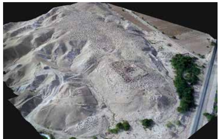
Figure 6. An oblique view of the drone-generated data displayed in 3D using ArcScene. By Austin (Chad) Hill, courtesy of Landscapes of the Dead project.
