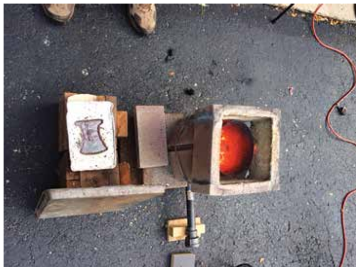
Copper poured into a plaster mold to make an ax head.
