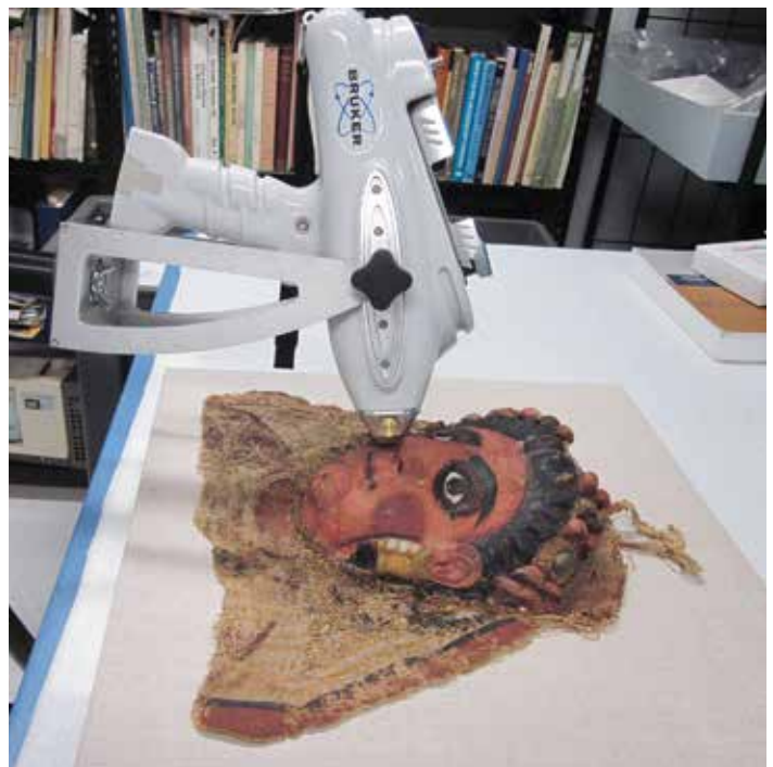
Figure 5. OIM E9385 undergoing XRF analysis.
