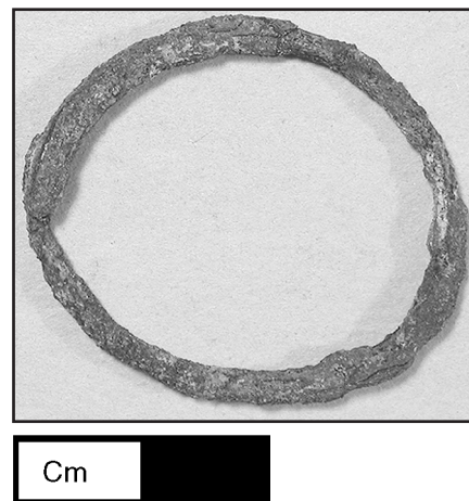
Figure 5. Copper alloy bracelet OIM A14136 from Megiddo, Israel, with unusual corrosion primarily in cracks in corrosion layers
